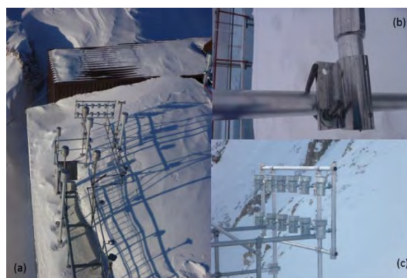
Figure 2: The “bird-feeders”/XAD-PAS from a bird-perspective (the weather mast) (a), the best approach outside (b), all twelve XAD-PAS deployed (c).
