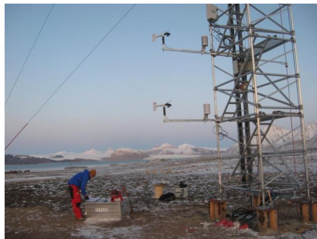
Photo 5: Setup near the surface of the lowest two meteo sensors
